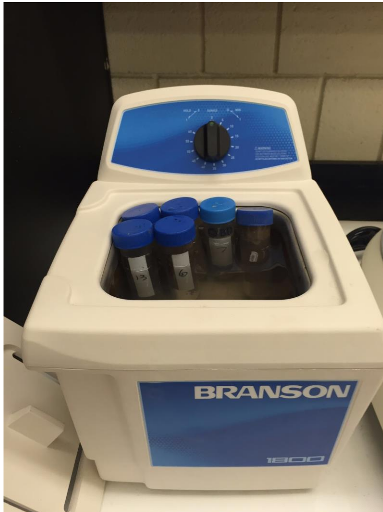
Figure 7: Ultrasonic cleaner to decrease surface tension and
