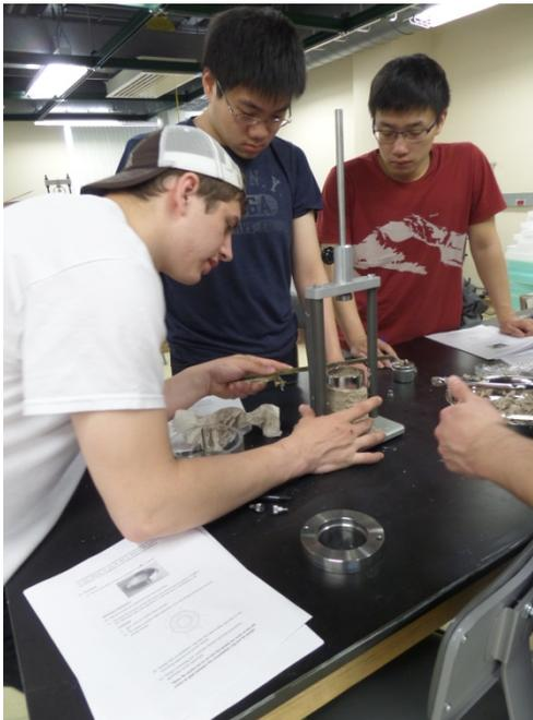
*Chris, Yuanchun, and Schicheng trimming a clay sample for a consolidation test.*
