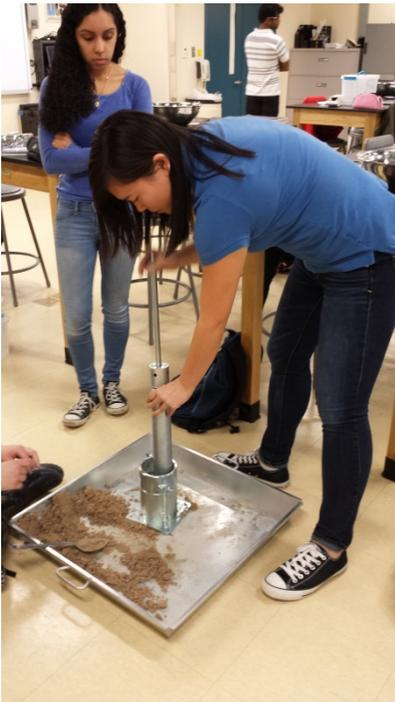
*Gabby and Emily working on a proctor compaction test in lab.*
